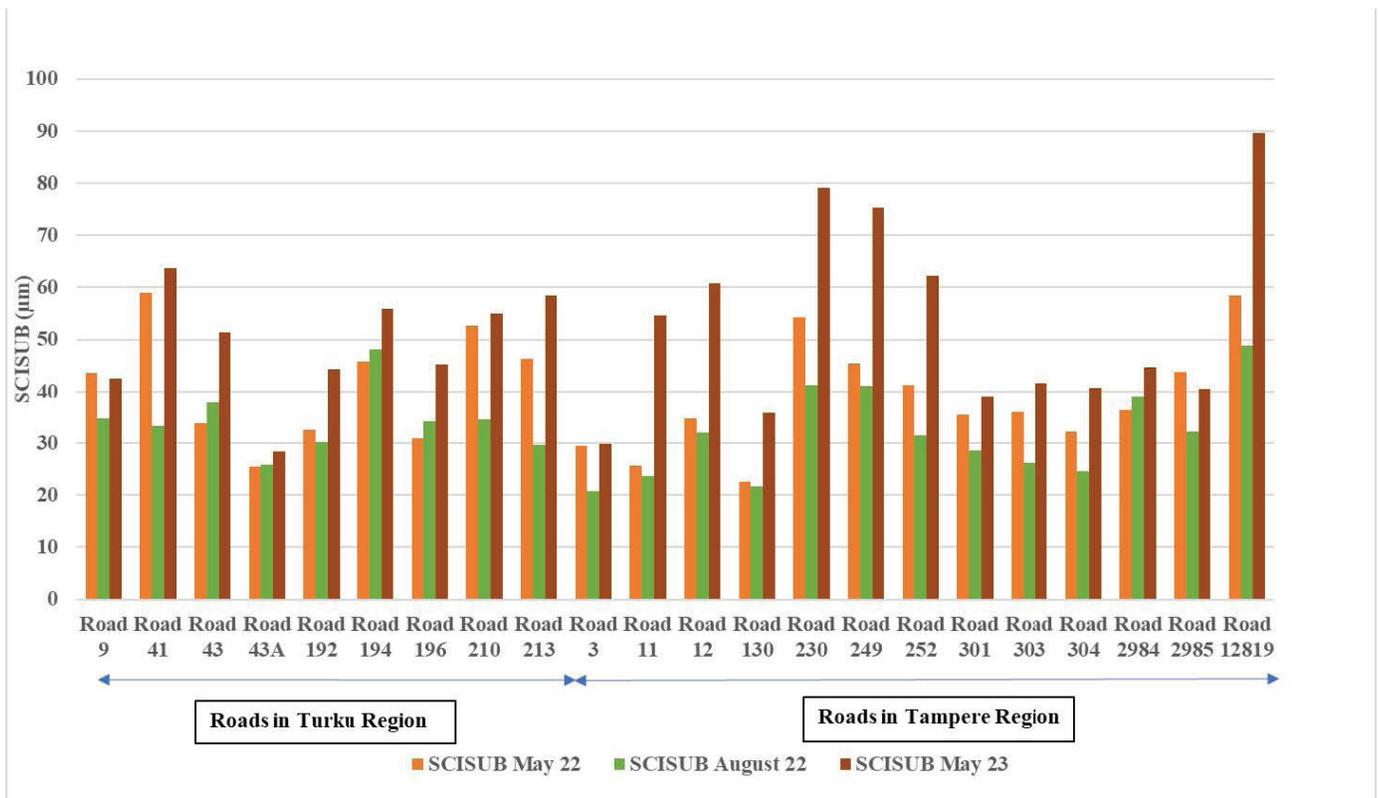
Figure 9. SCISUB calculated from measured deflections.
