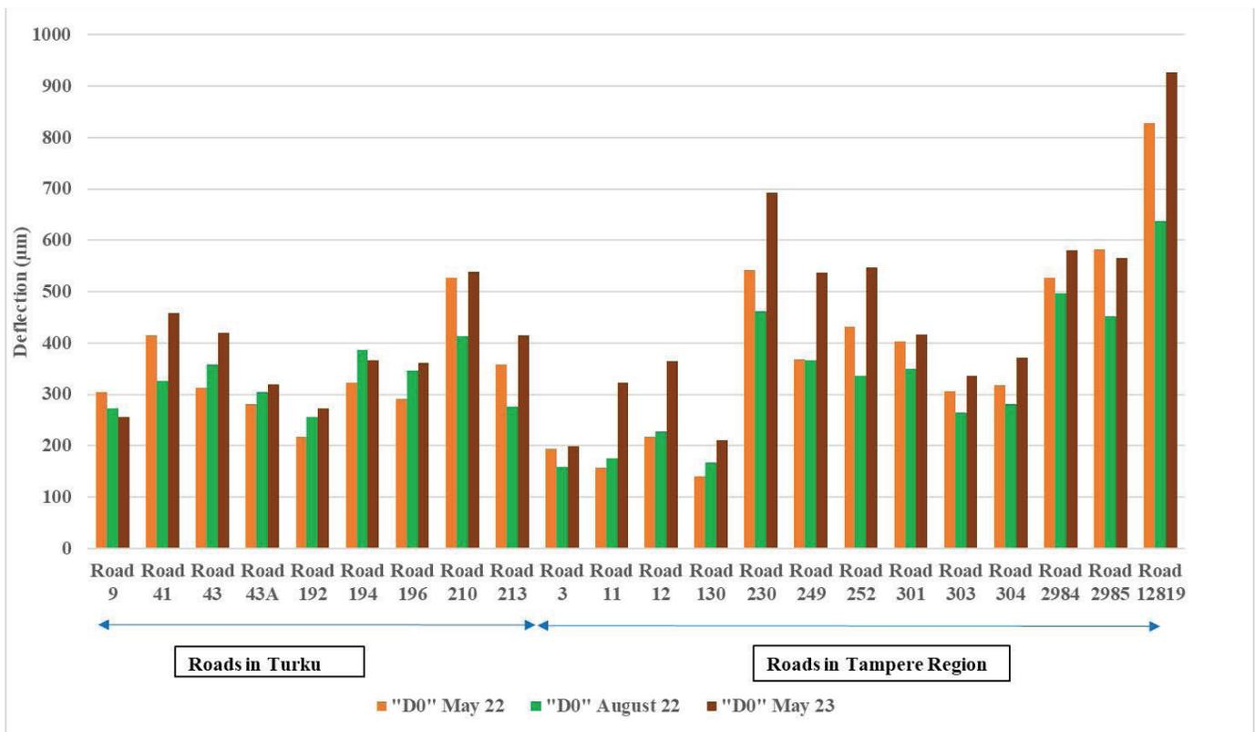
Figure 7. Center deflection measured by the iPAVe
