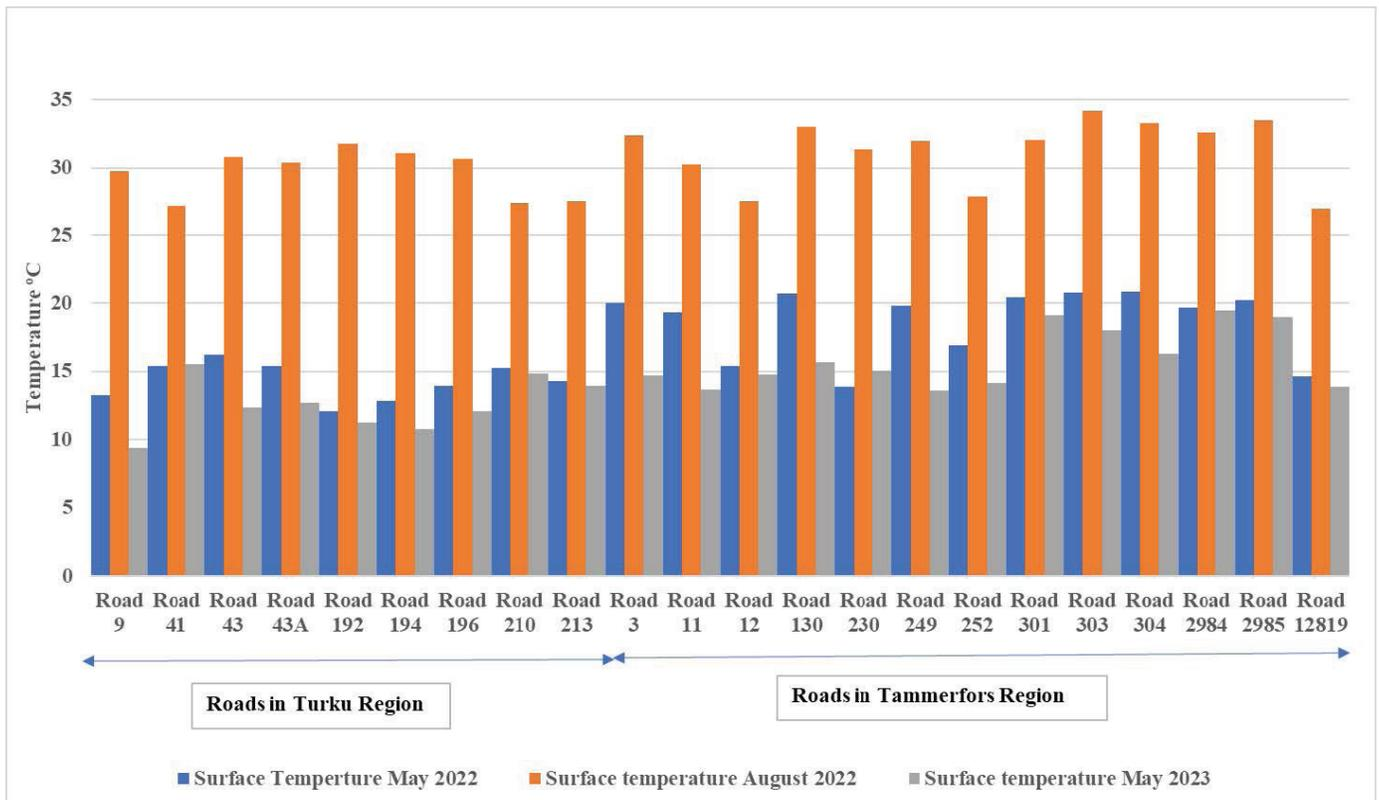
Figure 6. Average pavement surface temperature on each road measured by the iPAVE during condition measurements.
