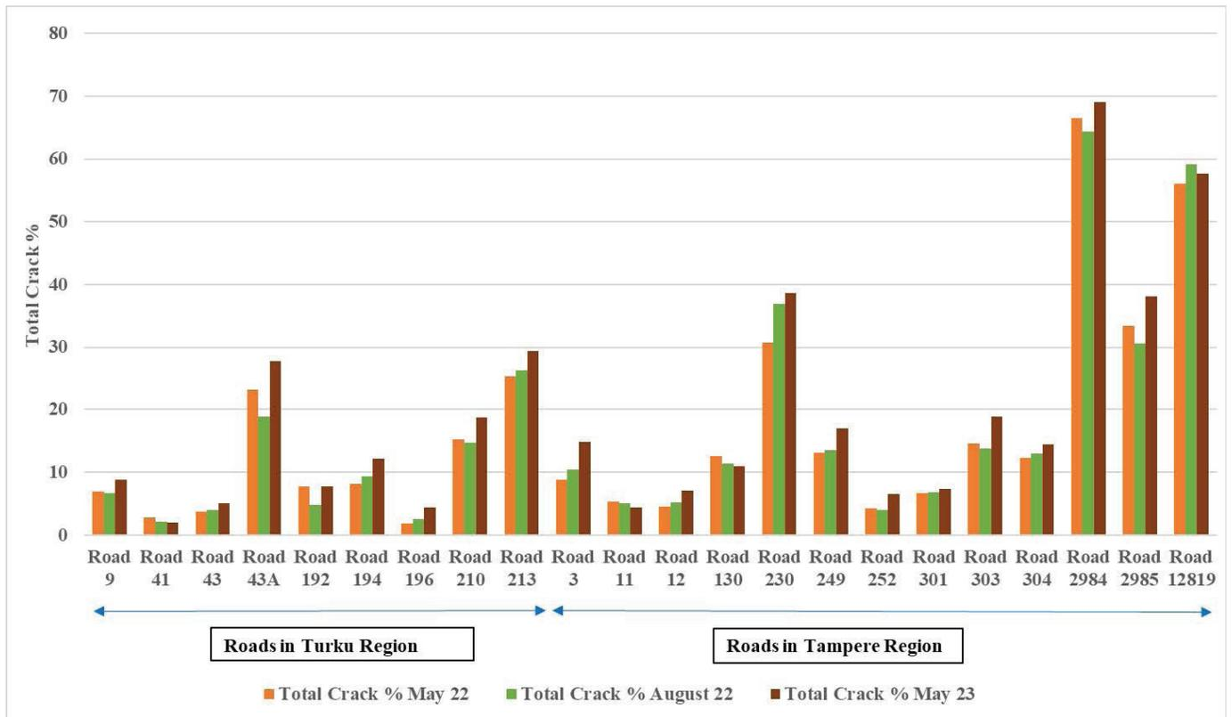
Figure 10. Total crack % of the pavements.
