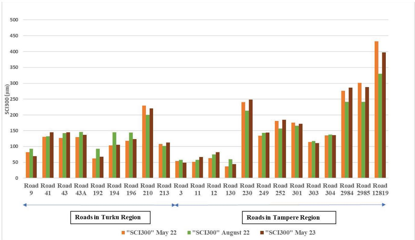
Figure 8. SCI300 calculated from measured deflections.
