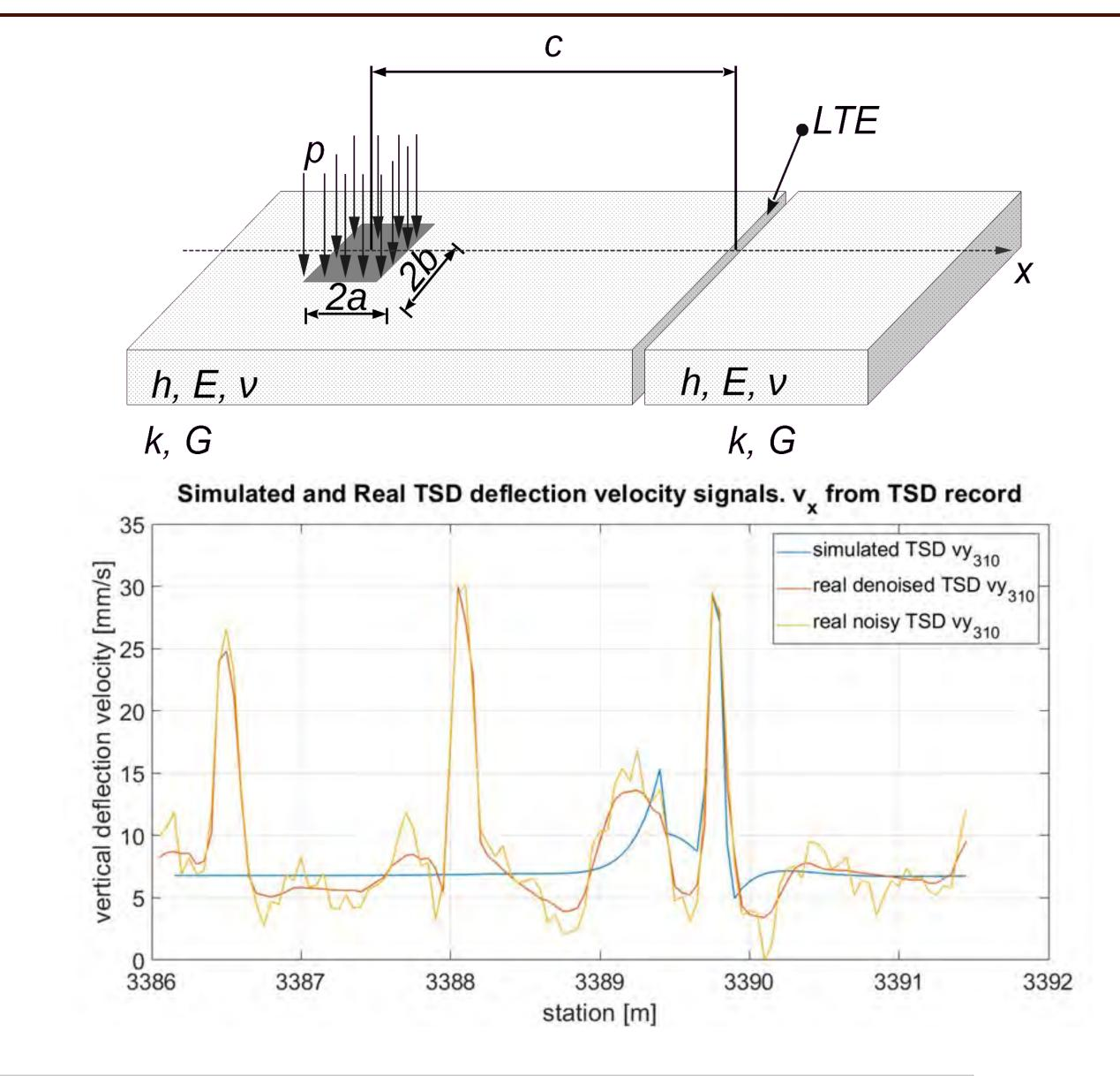
•We can back-calculate LTE of JPCP joints from TSD v<sub>y</sub> (4,6)
