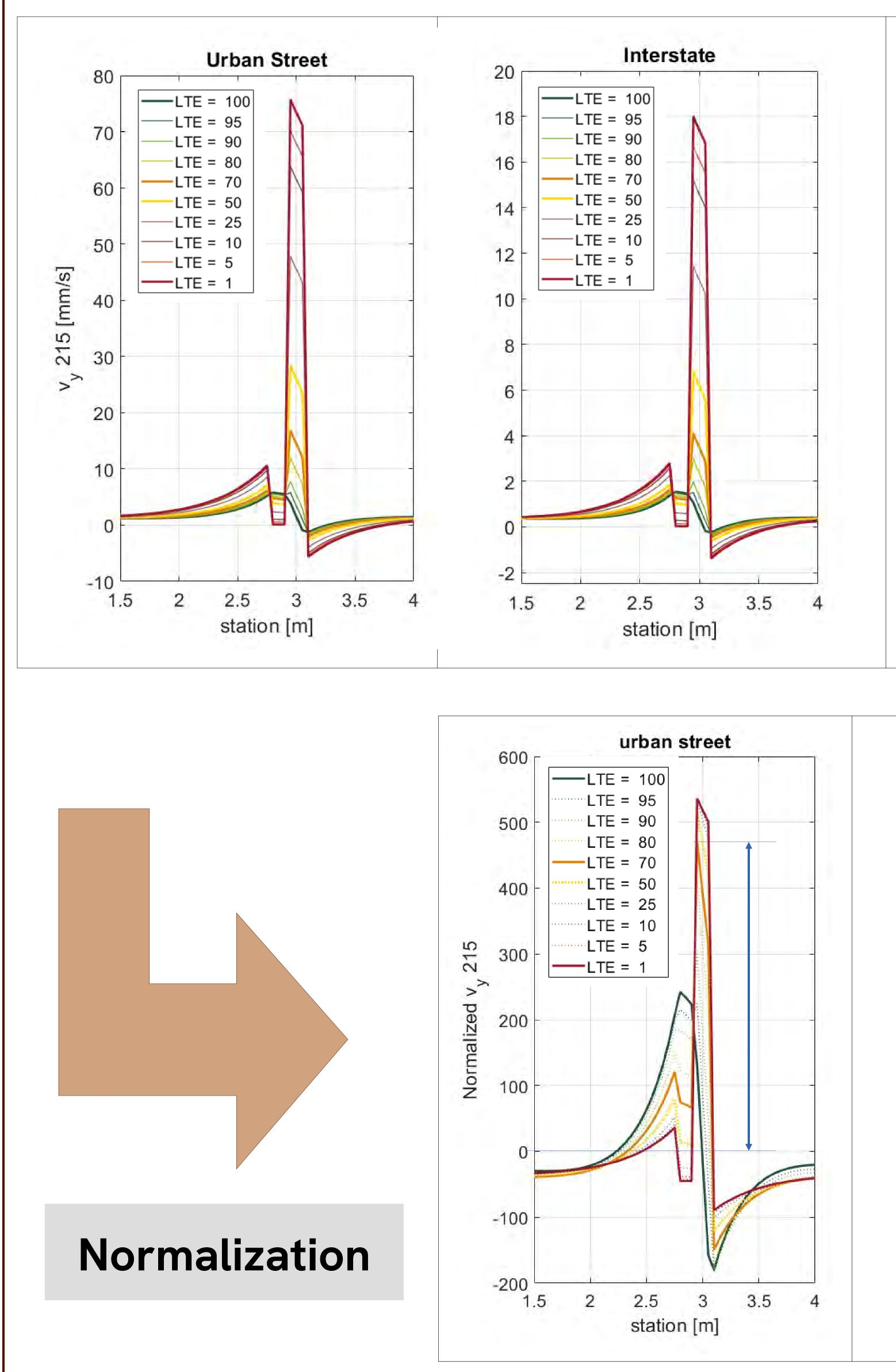
•All normalized  $v_y$ s reduce to a single set of shapes that vary with LTE,
