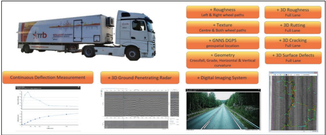
Figure 1: The intelligent Pavement Assessment Vehicle (iPAVe)
